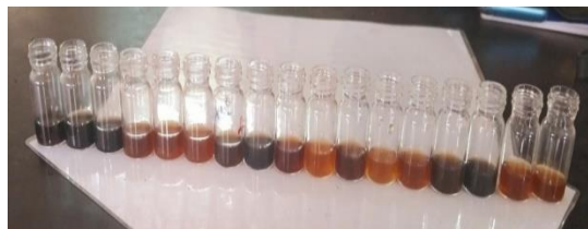
Fig. 2. Starch test observation for palmyrah jaggery market samples
